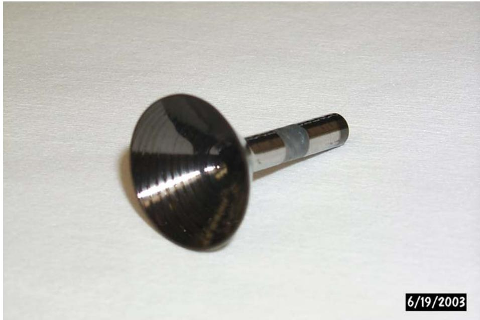
Figure 17. Quad Spiral Channel Electron Multiplier
