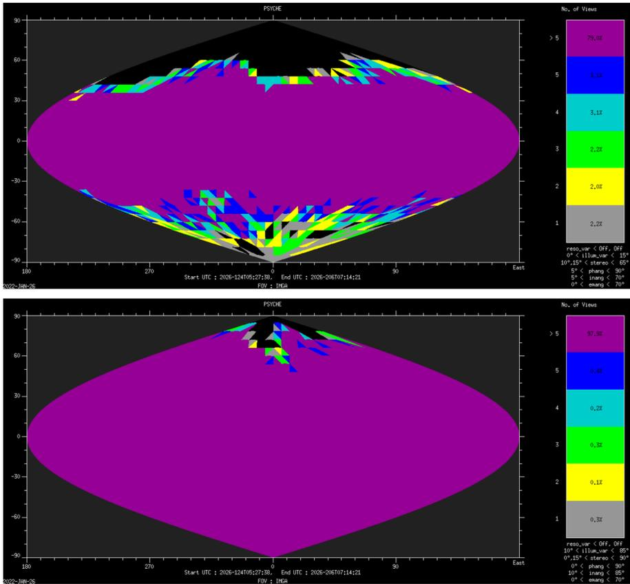
**Fig. 12** In Orbit B, SPG coverage meets the useable stereo conditions for incidence angle up to  $70^\circ$  (top) and resolutions of 10 m/pixel – 20 m/pixel. The bottom plot shows the coverage for SPC in Orbit B with the same resolution. The colors indicate the number of independent datums in each  $.25^\circ$  bin that collectively meet the criteria outlined in Table 1. The area covered at a given number of views is indicated by the percentage number in the legend
