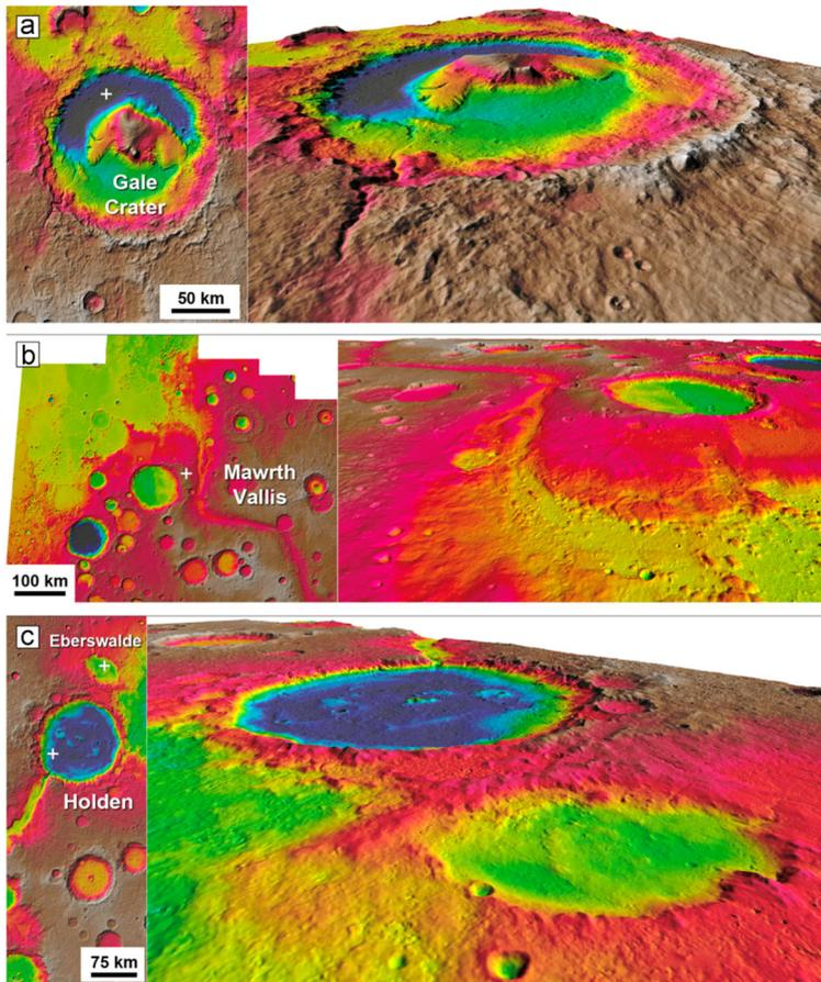
**Fig. 4** Examples of final DTM products. Mars Express HRSC multi-orbit DTMs of the final four candidate landing sites of the Curiosity (white crosses centers of proposed ellipses). On the left plan views (norths up); right-side perspective views; color-code elevations (red = high, blue = low). (a) Gale crater; (b) Mawrth Vallis; (c) Holden and Eberswalde craters (Gwinner et al. 2016)
