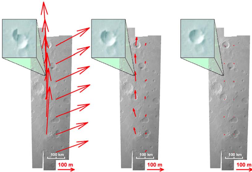
**Fig. 2** Example of displacements (red arrows). Identical points are identified in overlapping blocks of Mars Express HRSC images and corrected by bundle block adjustment (Gwinner et al. 2016)
