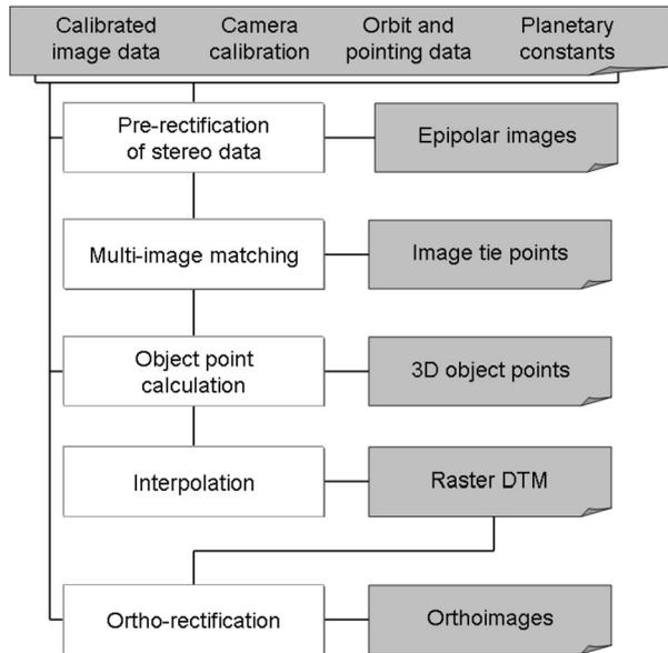
resulting in object points defined in body-fixed Cartesian coordinates. Multi-stereo capability enables minimization of the influence of occasional gross matching errors, which cannot be avoided by simple two-image matching.
