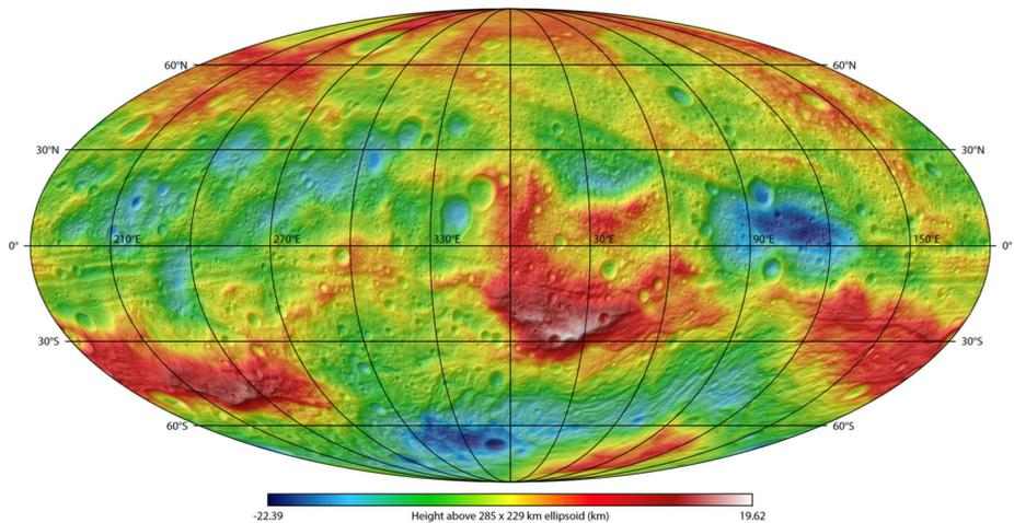
**Fig. 3** HAMO-based SPG-derived global topography of Vesta (e.g. Jaumann et al. 2012; Preusker et al. 2012, 2016) superposed on a hill shade model derived thereof. The map is in equal area Mollweide projection in the Claudia Double Prime reference system for Vesta (Li 2012)
