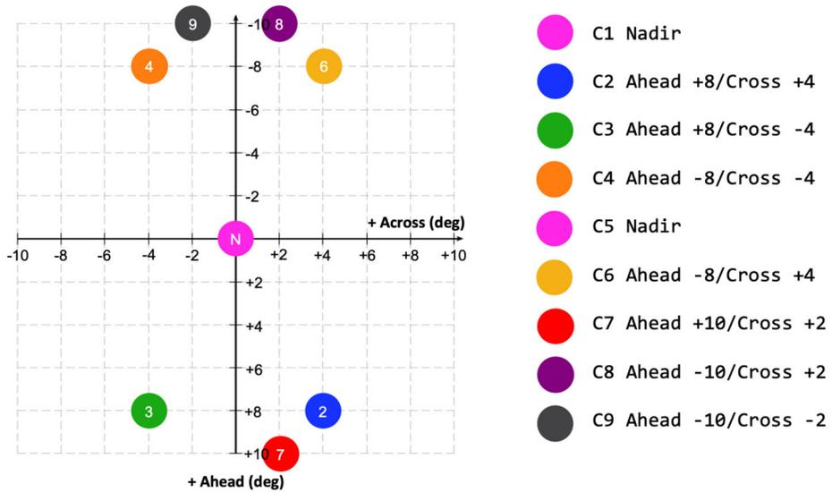
**Fig. 11** Illustration of the off nadir viewing geometry as referenced to spacecraft coordinates for the nine global mapping cycles (Polanskey et al. 2022). For a polar orbit, constant illumination is in the “Ahead” direction, while maximum illumination variation is achieved in the “Cross” direction. The angles in the Cross direction are maximized within the constraints of keeping on the body and achieving proper incidence and emission angles
