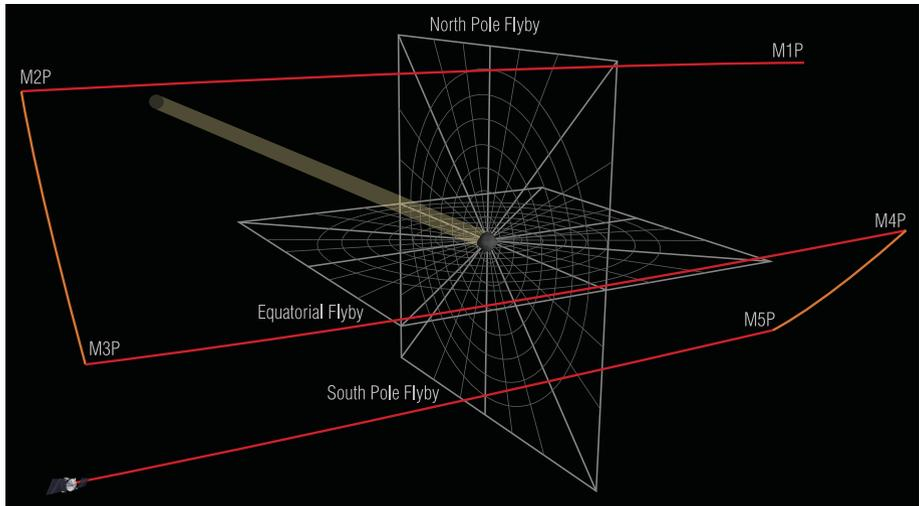
**Fig. 27** The OSIRIS-REx spacecraft's Preliminary Survey orbit path. The spacecraft will complete five legs to allow for flybys of Bennu's North Pole, Equator and South Pole, using trajectory changes at the Maneuver 1 Preliminary Survey (M1P) through Maneuver 5 Preliminary Survey (M5P) points
