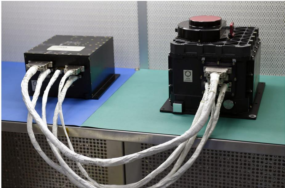
**Fig. 15** The Canadian Space Agency contributed the OSIRIS-REx Laser Altimeter (OLA), a scanning LIDAR (Light Detection and Ranging). OLA will emit laser pulses toward the surface of Bennu and measure the timing of the return pulses to compute the distance between the spacecraft and the surface of Bennu. OLA will use these data to provide high-resolution topographical information about Bennu during the mission (NASA)
