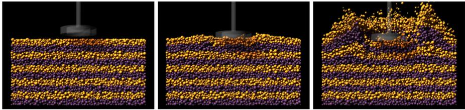
**Fig. 35** A model TAGSAM (visualized with some slight transparency) penetrates a bed of  $\sim 150,000$  particles (seen in cross section) with an initial downward vertical speed of 10 cm/s in the microgravity environment of Bennu ( $g = 20 \mu\text{m}/\text{s}^2$ ). The cylindrical container has a height and radius of 60 cm (Ballouz 2017 Ph.D. thesis)
