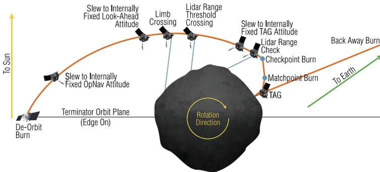
**Fig. 34** Diagram of the spacecraft’s Sample Acquisition trajectory, during which the spacecraft’s TAGSAM head will make contact with the asteroid Bennu to collect a sample of its regolith
