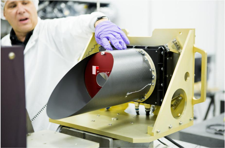
**Fig. 17** The OSIRIS-REx Thermal Emissions Spectrometer, provided by Arizona State University, determines mineral and temperature information by collecting infrared (from 5 to 50 microns) spectral data from Bennu (Arizona State University)
