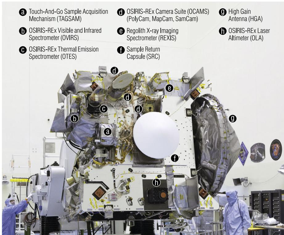
**Fig. 11** Labelled view of the OSIRIS-REx instrument deck. The spacecraft, mounted onto a rotation fixture in a NASA Kennedy Space Center cleanroom, has been rotated 90 degrees to place the instrument deck on its side (NASA)
