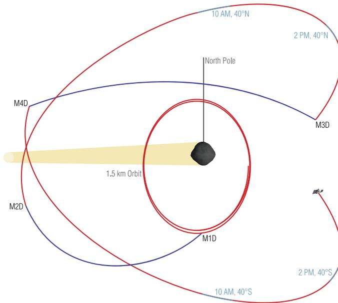
**Fig. 29** Trajectory diagram for the “Baseball Diamond” maneuver, which begins the mission’s Detailed Survey Phase. The spacecraft will progress through a series of hyperbolic passes around Benu, with trajectory changes at the Maneuver 1 Detailed Survey (M1D) through Maneuver 5 Detailed Survey (M5D) points
