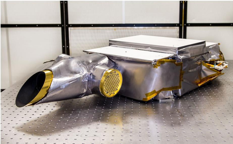
**Fig. 16** The OSIRIS-REx Visible and Infrared Spectrometer (OVIRS) will measure visible and near infrared light from Bennu, which can be used to identify water and organic materials on the asteroid. OVIRS was provided by NASA Goddard Space Flight Center (NASA)
