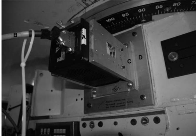
FIG. 6.—A PHOT camera (MicroMax 512BFT) mounted on the auxiliary port of the 3.9 m AAT. Shown here are the MicroMax CCD head unit (a), the cable (b) connecting it to the electronics box, the aluminum standoffs to which the camera is bolted (c), and an adapter plate (d) with a bolt hole pattern to mate the standoff unit to the telescope.
