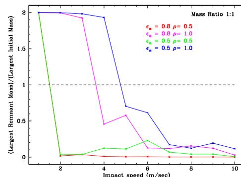
FIGURE 3: High-resolution equal-mass collision accretion values as a function of impact speed for the four cases of bulk density and coefficient of restitution. The plot shows the sharp cutoff between accretion and erosion as a function of velocity.
